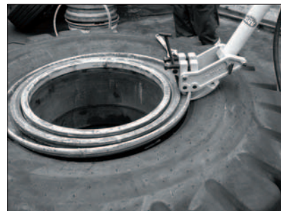
Hydraulic tire remover (tire push type) in operation
